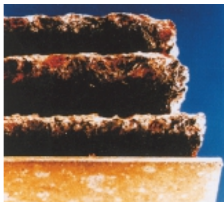
經在工業區曝露17年之端面外觀 Edge Appearance of Coated Sheet After About 17 Years Industrial Exposure (Bethlehem.PA.U.S.A)
